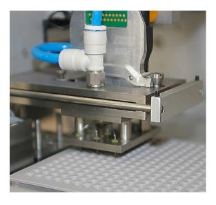
Figure 2. JetSpyder™ penetrating through JetGuard™ to access samples without exposing them to the atmosphere
