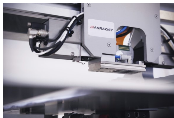
Figure 1: Twin cameras sit either side of the print head and comprise the Iris™ Optical QC System which captures images of printed slides within 300 ms of sample deposition.
